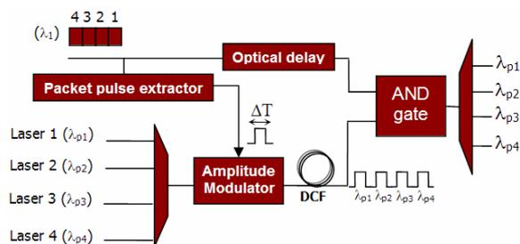
Figure 2- Schematic diagram of a 4-bit time-to-wavelength converter
